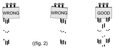
Basically, you are trying to distribute the same amount of water to all the eight holes equally. Once you level head you may need to add a little more water by slightly opening the flow valve a little more. The change will not be immediate. Flow changes should be slight. To much flow will cause water to flow from the four breather holes located on the bottom of the head.
